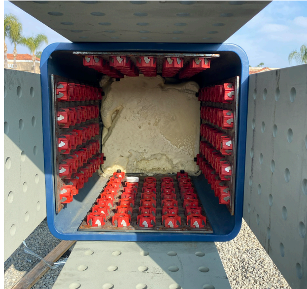
An HSS 22x22x7/8 set up for a bolted splice using Shuriken.
