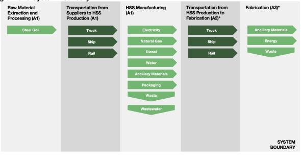
All A1 steps represent manufacturing of unfabricated HSS by Atlas Tube. Stages with an asterisk rely on data from the AISC & STI industry average EPD for fabricated HSS (AISC & STI, 2022). This EPD does not declare the modes of transportation used in A2, so it is assumed all common modes (truck, ship, rail) are used.
